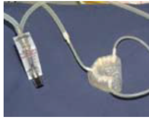
Figure 2: Ozone gas is sucked into the bleach guard through tube on the left and extracted via the two tubes on the right. Extracted ozone gas went through the flow meter to the suction pump in the Ozicure treatments. The flow meter regulated the removal of the ozone gas from the guard that covered the teeth in the base model. The ozone gas was extracted at a rate of 5l/min.
